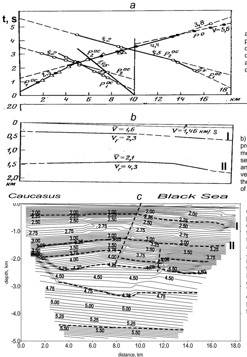
a) Traveltime curves along profile 22 with designations of head waves and values of apparent velocity according to interpretation of 70s years.
